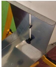
3. This is to adjust the height of the hopper for easier loading.
