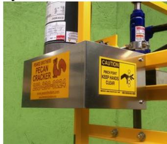
6. Do not operate the machine with guards missing.
