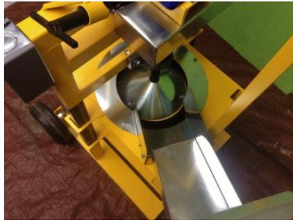
3. Plug the hopper into the GFCI receptacle on the cracker. Place a tote under the cracker to catch the pecans.
