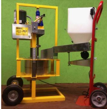
2. Roll the cracker in place and align the hopper feeder chute with the funnel on the cracker.
