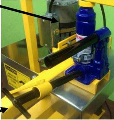
2. **This handle**, when turned counter clock wise, lowers the cracker cage for smaller pecans. It must be turned clockwise to stop lowering the cage. Be careful not to over tighten. This could damage the jack.
